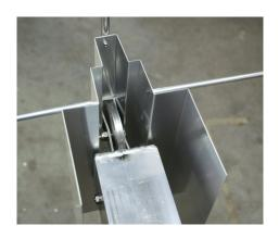
STEP 7: Thread the winch handle onto the winch. Slide the spring onto the winch beside the handle. Secure the spring with the <sup>3</sup>/<sub>4</sub>" wide nut.
