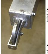
**STEP 3:** Insert the aluminum pulley into the pulley assembly located on top of the pole. Insert the 5/16" x 1-1/4" bolt through the assembly and pulley, secure with 5/16" lock nut.
