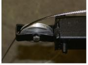
STEP 6: Feed the cable through the top plastic glide and through the pulley at the top of the pole. The cable can not be twisted around the pole.
