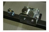
STEP 11: Feed the cable through the small pulley. This small pulley will keep the cable close to the pole and aliened with the bottom plastic guide.
