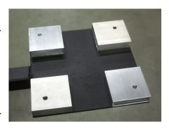
STEP 16: Place one 2-1/4" x 4-1/2" aluminum plate inside each of the four bottom compartments aligning the holes. This plate is for adding stability to the floor.
