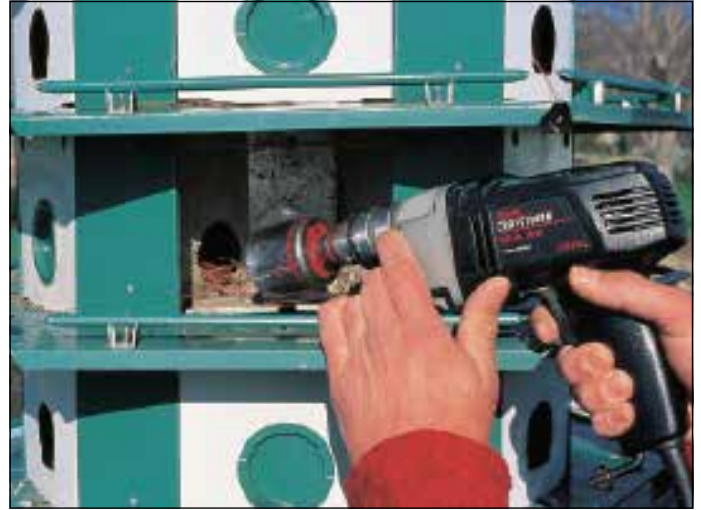
Fig. 5. A modified Trio-Castle (PMC-24CP). Compartments were enlarged, in position, by drilling a 2-inch hole through every other interior wall partition, then plugging every other entrance hole with door stops.
