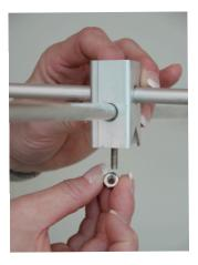
• Pole with diameter of 1-1/4": After sliding perching rods through notched mounting tube, position white PVC cap under notch with the open end of the tube facing downward. Drop the stainless steel bolt through all holes and secure with nut. Slide over the top of the pole. Tighten the embedded setscrew with the supplied Allen wrench to secure it to the pole.
