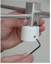
• Pole with diameter larger than 1-1/4": A bolt measuring at least 3" long will need to be purchased separately. Remove the existing pipe cap and drill a 3/16" hole in the center of its top. Thread the bolt through the holes in the perching rods and PVC cap and into the pipe cap of the pole. Tighten the nut and place the entire assembly back on the top of the pole.
