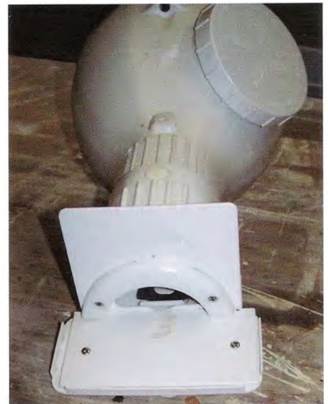
A slight groove was filed in the raised porch, matching the bottom center dip of the Conley II entrance. If the raised porch does not come up enough to block the bottom of the Conley II, no groove will be needed.
