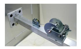
**STEP 12:** Wind the cable end into the side of winch. After winding the cable, insert the cable end into the cable stop that is provided. Using a pliers or channel locks, pinch the cable stop enough to keep the stop from sliding off of the cable. This stop is to keep the cable end from fraying.
