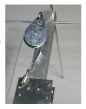
**Step 9:** When raising your housing, some types may actually hit the top perch rods and bend them. To prevent this from happening, attach the two 3-1/2" aluminum plates to the pole using two 1/4" x 2-3/4" bolts with flange nuts. The stop should be mounted above the hub and adjusted according to the height of your martin houses.
