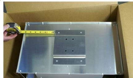
**Method A; Step 3:** Drill 1/4" holes at the marked locations. Repeat this process for the remaining martin house.
