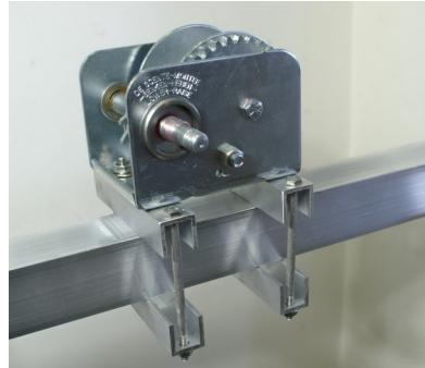
**Step 9:** Attach the cable guide pulley approximately 10" above the winch using one aluminum u-channel and 1/4 x 4-1/2" bolts and flange nuts.
