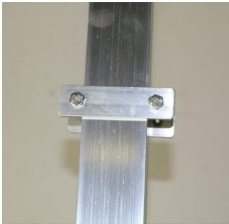
**Step 8:** It is important to mount the winch on the same side of the pole as what the cable that extends downward. Mount the winch using two aluminum u-channels and 1/4" x 4-1/2" bolts with flange nuts. The winch can be mounted at any desired height though nest checks will be easier if the winch is mounted lower to the ground.
