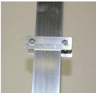
**Step 8:** It is important to mount the winch on the same side of the pole as what the cable that extends downward. Mount the winch using two aluminum u-channels and 1/4" x 4-1/2" bolts with flange nuts. The winch can be mounted at any desired height though nest checks will be easier if the winch is mounted lower to the ground.
