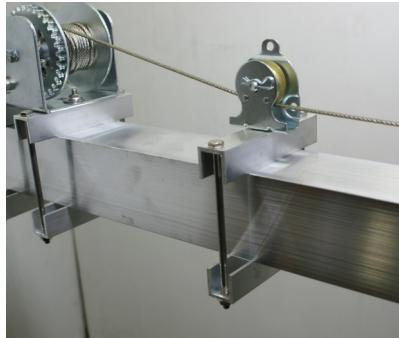
**Step 10:** Thread the winch handle onto the winch. Slide the spring onto the winch beside the handle. Secure the spring with the 3/4" wide nut.
