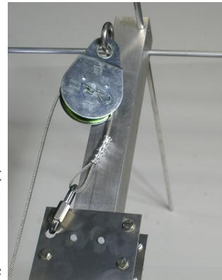
**Step 7:** When raising your housing, some types may actually hit the top perch rods and bend them. To prevent this from happening, attach the two 3-1/2" aluminum plates to the pole using two 1/4" x 2-3/4" bolts with flange nuts. The stop should be mounted above the hub and adjusted according to the height of your martin house.
