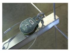
3" angle attached to the hub) is at the top . Insert the bottom end of the pole into the top end of the hub and slide the hub upwards to the top of the pole.
