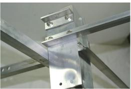
STEP 3: Attach the four long pieces of aluminum angle to the hub as shown.
