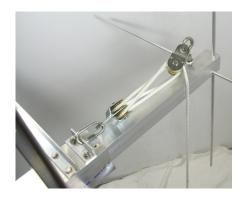
STEP 8: Remove the locknut from the eyebolt and insert the eyebolt into the remaining 3/8" hole at the top of the pole (See photo). The split, in the eye, of the eyebolt should be turned upward so the pulley will hang freely and the eyebolt will not open with the weight of the hub. Reattach the locknut and tighten with wrench.
