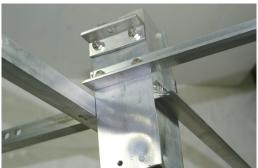
STEP 3: Attach the four long pieces of aluminum angle to the hub as shown. The holes in the hub are threaded. Use eight 1/4 x 1/2 bolts with 1/4" lock washers. The angle is turned with the flat side being turned down so that martins can perch on the angle arms.
