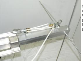
STEP 5: Orient the pole so that the remaining hole, at the top of the pole, is vertical and on the left half side of the pole as shown in the photo. Orient the hub so the quick link, double pulley and rope is at the top left hand corner. Insert the bottom end of the pole into the top end of the hub. Slide the hub upward to the top end of the pole.
