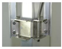
STEP13: Vertically hung gourds may require their hanging holes to be enlarged to 3/8". Slide the gourd onto the arm and insert a hitch pin into the small hole, at the end of the arm, to keep the gourd from sliding off.
