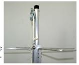
STEP 7: Attach the rope winder to the pole using 1-3/4" bolts and hex nuts. The rope winder should be attached on the same side of pole as the pulley at the top to assure proper alignment for the rope. The rope winder can be placed at any height that is comfortable.
