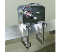
STEP 12: Thread the winch handle onto the winch. Slide the spring onto the winch beside the handle. Secure the spring with the 3/4" wide nut. (See picture on left)
