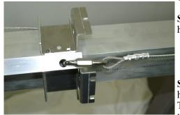
STEP 10: Insert the quick link found in your hardware bag into the 1/2" hole and attach the cable loop. Close the quick link and tighten with wrench.
