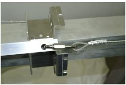
**STEP 10:** Insert the quick link found in your hardware bag into the 1/2" hole and attach the cable loop. Close the quick link and tighten with wrench.
