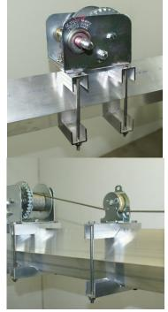
**STEP 13**: Thread the winch handle onto the winch. Slide the spring onto the winch beside the handle. Secure the spring with the  $\frac{3}{4}$ " wide nut. (See picture on left)
