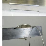
STEP 8: Place a stop bolt which is  $1/4 \ge 3-3/4$ " into the remaining hole and secure with
