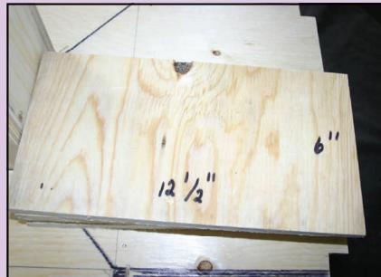
***Measure and cut the middle divider for the third floor.***
