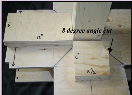
**After notching the second floor and third floor corners , nail the second floor to the dividers on the lower level using one inch galvanized nails. Measure and cut the divider pieces for the second floor.**
