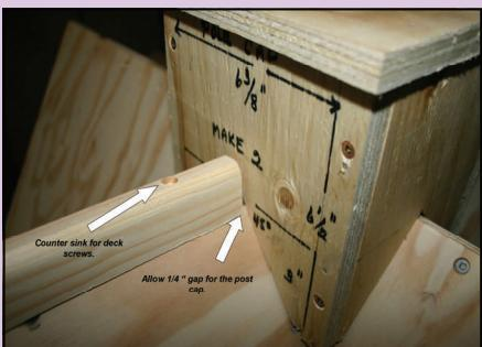
*Roof ridge has been fastened into position with post cap in place.*
