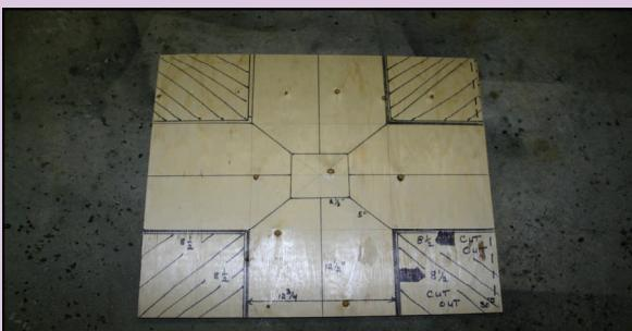
*Use the similar format for cutting out the 30"x 30" panel. The area to be cut out should measure 8 1/2" x 8 1/2".*
