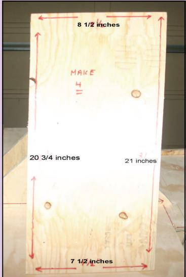
*Cut 4 identical pieces of 1/2 inch plywood for the sides ensuring that the good side faces out.*
