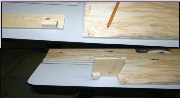
*Construct a jig using a piece of 1/2 inch plywood and pine stock 3/4 " x 1". This will be used to mark out the corners of the second and third floors after removing excess material.*
