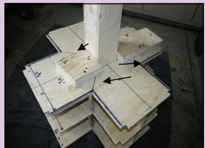
***Nail the third floor to the second floor dividers and measure and cut the dividers for the third floor.***
