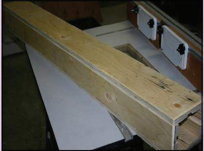
*Nail and assemble the sides of the pole shaft using 1 1/2" galvanized nails. The inside dimension of the tube should accommodate a 4" x 4" (3 1/2" x 3 1/2") standard wooden pole or a 3" o. d. round or square metal pole.*
