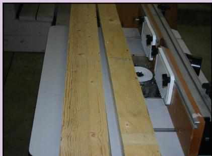
*Cut 4 pieces of 5/8" plywood ( 36"-48") long to allow for a 3 3/4 " clearance inside the tube section.
