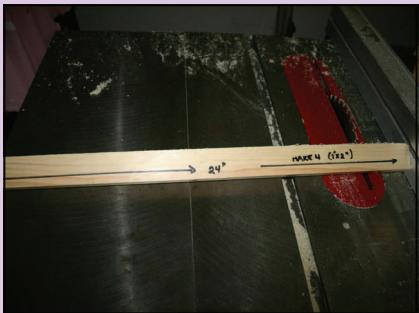
*Make four roof ridge caps from an 8 'x 1" x 2" inch pine piece. Each piece should measure 24 " long .*
