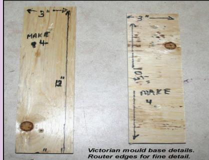
*The Victorian fretwork bracket is comprised of three pieces- the bracket and two pieces of supporting 1/2 inch plywood. Cut out your bracket from 2 inch MDF or pine. Rout the pieces to create a smooth edge before assembling and painting. Cut out the plywood pieces as indicated.*
