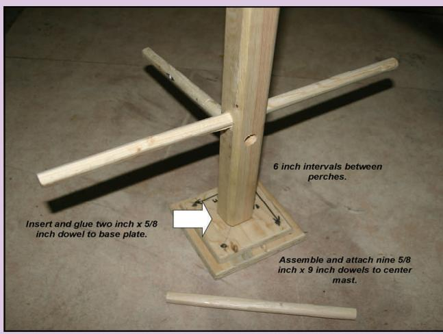
*Construct the mast from pine. The measurements of the center mast are 2"x 2" x 36". Rout the edges of the mast with a round over bit. Drill 5/8 inch holes on opposite sides of the mast at 6 inch intervals.*
