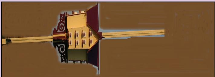
*Slide the house on the pole and slide the cable through the slot in the post tube over the pulley and secure the end to the bottom of the house. Have someone help you!*
