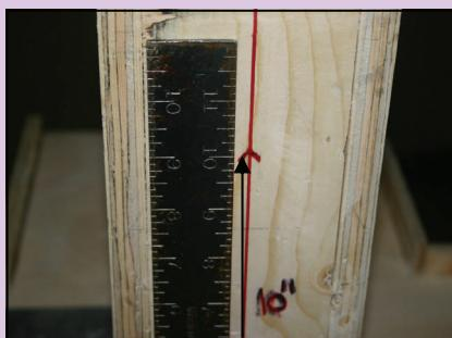
*Measure and mark 10 "from the base to the top of the pole.*
