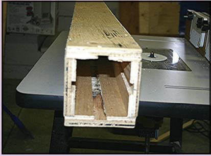
*The completed and assembled pole shaft illustrates the grooves on the inside of the pole to accommodate any cable configuration . N. B. Use a piece of 4"x 4" and test your tube before proceeding.*
