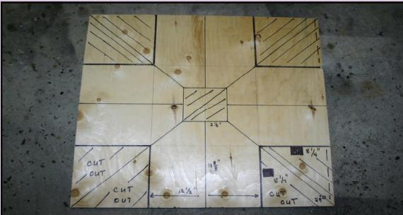
*Using the same format as for the previous piece mark out the details for the 29"x 29" piece. The area to be cut out should measure 8 1/4"x 8 1/4"*
