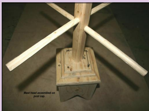
*The mast piece may be attached with four drywall screws. The completed mast head is ready to be sanded and painted.*
