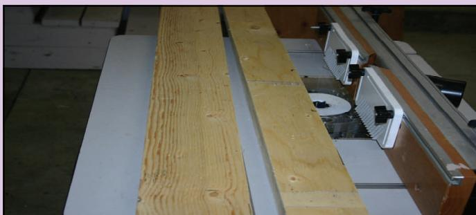
*Select the smooth crown side of the plywood for routing the cable path.*
