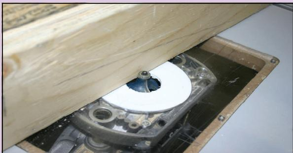
*A 1/4" round over bit is used to smooth the outside and inside edges.*
