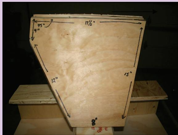
**Similarly, cut four pieces according to the following illustration. Angle cut the top section at 45 degrees. Ensure that the good side of the plywood is facing outward.**
