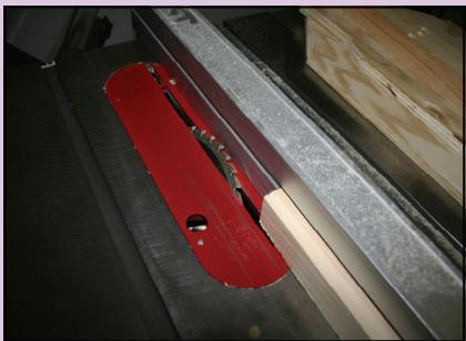
*Set your saw on a 45 degree angle and run your pine to form a 45 degree v-groove on the bottom of each piece.*
