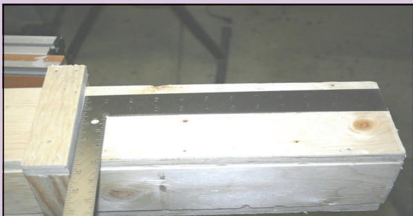
*Position the pieces 12 inches from the bottom of the pole shaft. The cleat on the bottom can be used later to attach your cable.*
