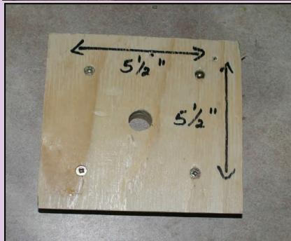
*Mast assembly pieces are constructed from two pieces of 1/2 inch plywood:*
