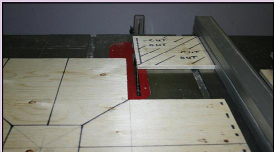
*On all plywood remove each of the corner sections as marked. Once the fence on the table saw is fixed at the correct measurement i.e. 8" then all corners can be removed exactly. Make a single cut first measuring 8".*
