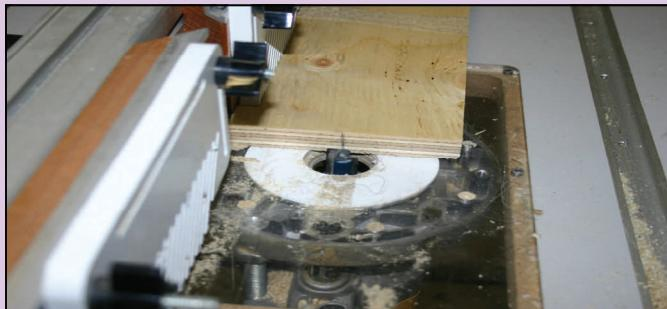
*Center the router bit to make sure the router path is directly in the center of the post sides.*
