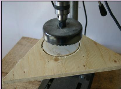
***Cut out 16 discs using a 5 inch hole cutter from 1/2 inch stock.
