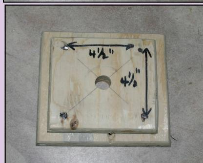
*Assemble the two pieces with drywall screws and drill a 5/8 inch hole in the center to center the mast pole dowel. Rout the edges of each piece.*
