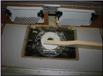
*A router can be used to round over the top edges and shape the end piece.*
