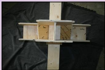
**Assemble and nail the pieces as illustrated using 1" galvanized nails. Toe nail the side dividers into the main post tube. Make sure that the dividers are flush to the side walls. Add the second floor and prepare to nail the dividers from the top.**
