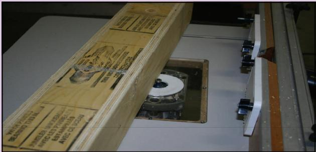
*Set up your router to accommodate the corner edge of the post shaft.*
