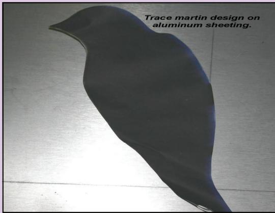
*Using a template trace the image on a piece of galvanized metal sheet or aluminum. Use a punch to detail the eyes.*
