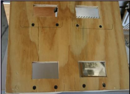
*Measure and screw the disks to each of the front pieces allowing a 1/8"- 1 " space below the entrance hole. If starling resistant plates will be used the porches should be placed as close to flush with the hole as possible but 1/4"- 1/2" is often recommended.*
