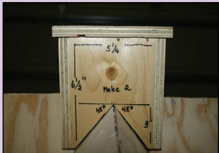
***The pole cap is constructed of 3/4 “ material and consists of four sections and a cap. Mark and cut out two pieces as illustrated.***
