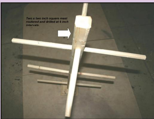
*The dowel pieces have been glued and a brad nail used for each perch to secure it to the mast..*
