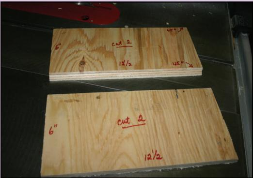
**Cut and preassemble the following pairs of dividers and roof panels. These will be used just below the roof section. The upper piece in the photo will be angled cut at a 45 degree angle to accommodate the roof slope.**
