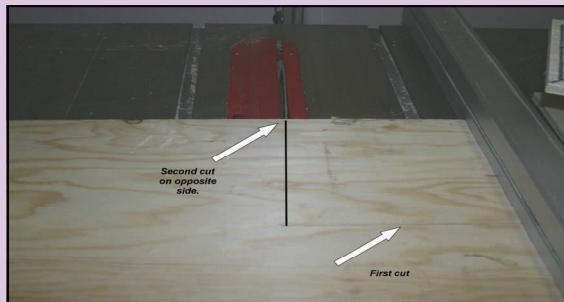
*Turn the plywood piece over and make another 8" cut. Repeat the process until all corners are removed.*
