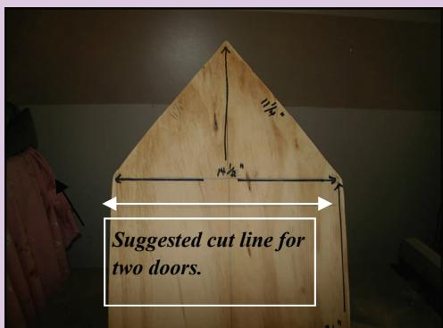
*The front door piece may be left in one piece or cut in two to allow for a free swinging door. Cut the door 1 inch below the upper floor level so it can be opened.*
