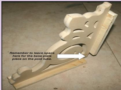
*The fretwork is now assembled and ready for painting. Adjust your fretwork to the bottom plate of the house before assembling. Do not attach the fretwork until your house is mounted on the pole.*
