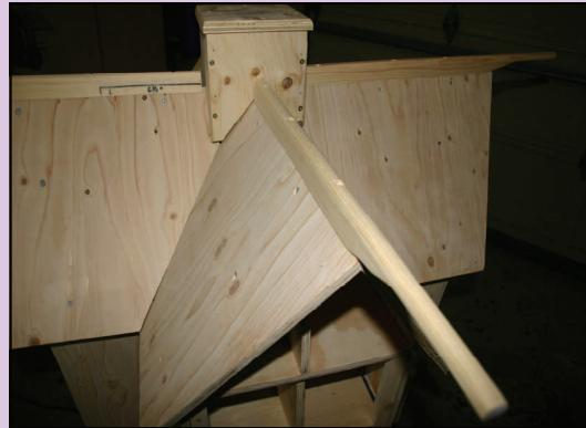
*Measure and cut four pieces of 1/2 inch good one side plywood for the front pieces according to the measurements as illustrated.*
