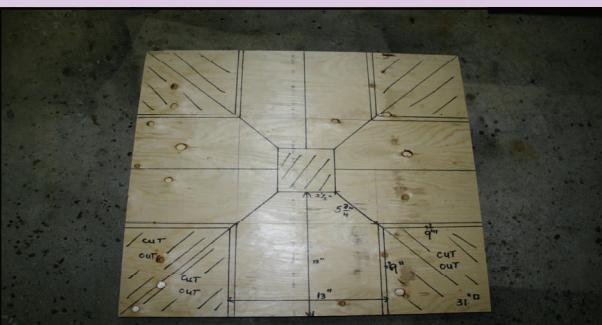
*Finally measure and layout the 31"x 31" panel. The area to be cut out should measure 8 3/4"x 8 3/4".*
