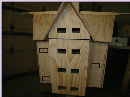
*The entrances have been cut out to accommodate starling resistant plates. Round /SRE holes can be cut directly into the wood if preferred. Note the possible placement of entrances on the sides as well.*
