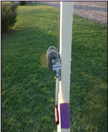
***Lower the martin house so it is at its lowest level and then slowly raise the martin house into position. Make sure the pulley is turning at the top of the pole. Do not raise the house too high to bind the pulley and lift off the post cap!***
