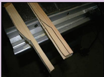
*Contour cut the end of the pine piece to allow for some architectural variance using a jig or band saw.*
