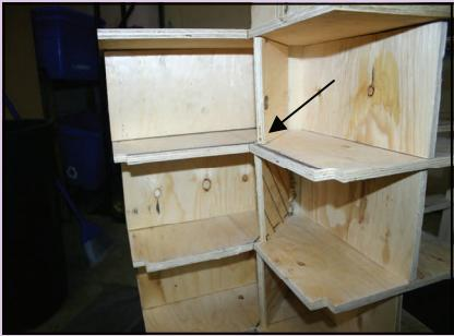
*The dividers should be positioned so they do not interfere with the installation of the side walls. They should be set flush to the floor edge.*
