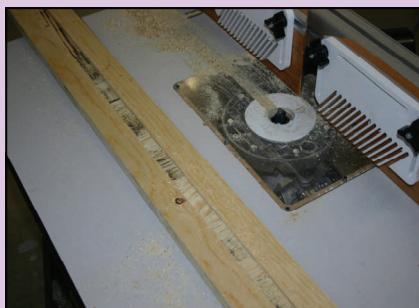
*Rout a path 1/2" wide and 3/8" deep along the center length of all pieces. This will be used later to accommodate the cable which will run the length of the pole.*
