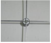
**Step 5:** Slide the top cap onto the top end of the pole as shown in photo. Top cap is held by friction.
