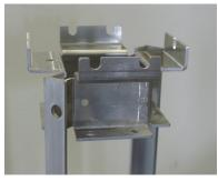
When you complete the hub, you should be able to look down one side of the hub and see alternating numbers of u-shaped notches in each row (see photo). Tighten all bolts securely.
